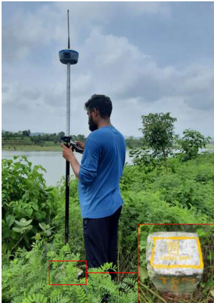
Figure 3.2: Temporary Benchmark 2 (LAKHI DAM TBM2)
