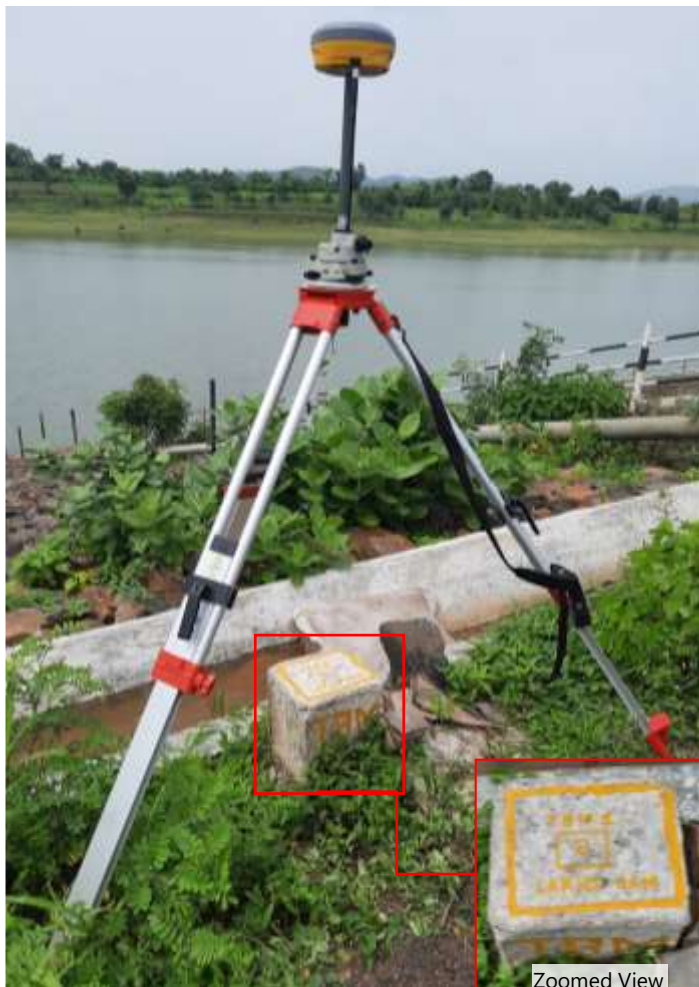
Figure 3.1: Temporary Benchmark 1 (LAKHI DAM TBM1)
